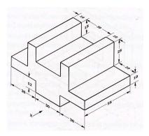
10.Draw the front view, top view and left side view of the object shown in the fig.
