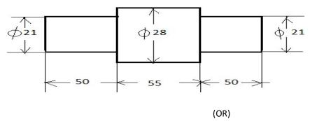
Estimate the number of rivets made from 4.5kg of mild steel as shown in the density of the material is 7.87 grams/cm3. All dimensions are in mm.
